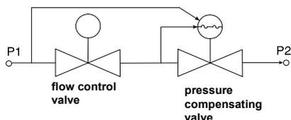
For process conditions where up- and downstream pressure varies much, a special type of valve, VARY-P has been designed. This valve consists of two valves, a solenoid operated control valve and a fixed adjusted pressure compensation valve.
