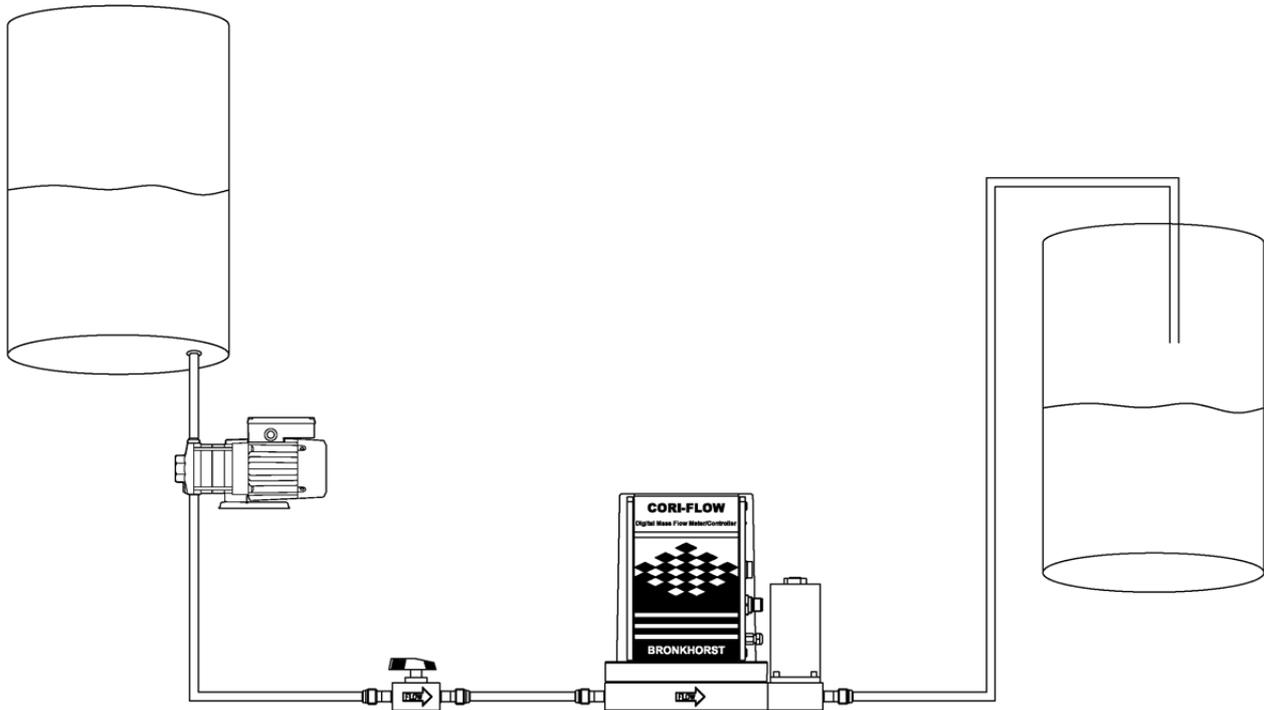
Install the sensor up side down in horizontal position for low flow (< 1000gr/h Full Scale) liquid measurement (see the following figure) and horizontal straight up for higher liquid flows and gas measurement.
