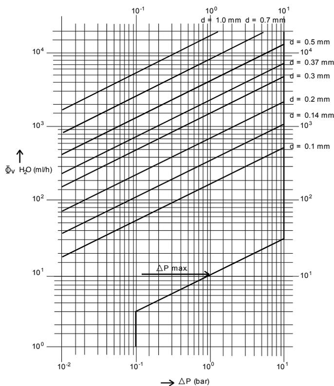
If liquids have viscosity's >15 cs (water = 1 cs), the flat orifice and plunger type control mechanism cannot be used. For measuring systems only check maximum possible viscosity with factory.
