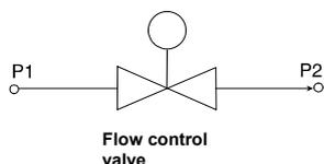
This is considered to be the standard (direct operated) control valve. In general it is a normally closed solenoid valve. The plunger is lifted by the force of the magnetic field of the coil. The orifice under the plunger is removable for optimising the orifice diameter. Also a normally opened solenoid valve is available.
