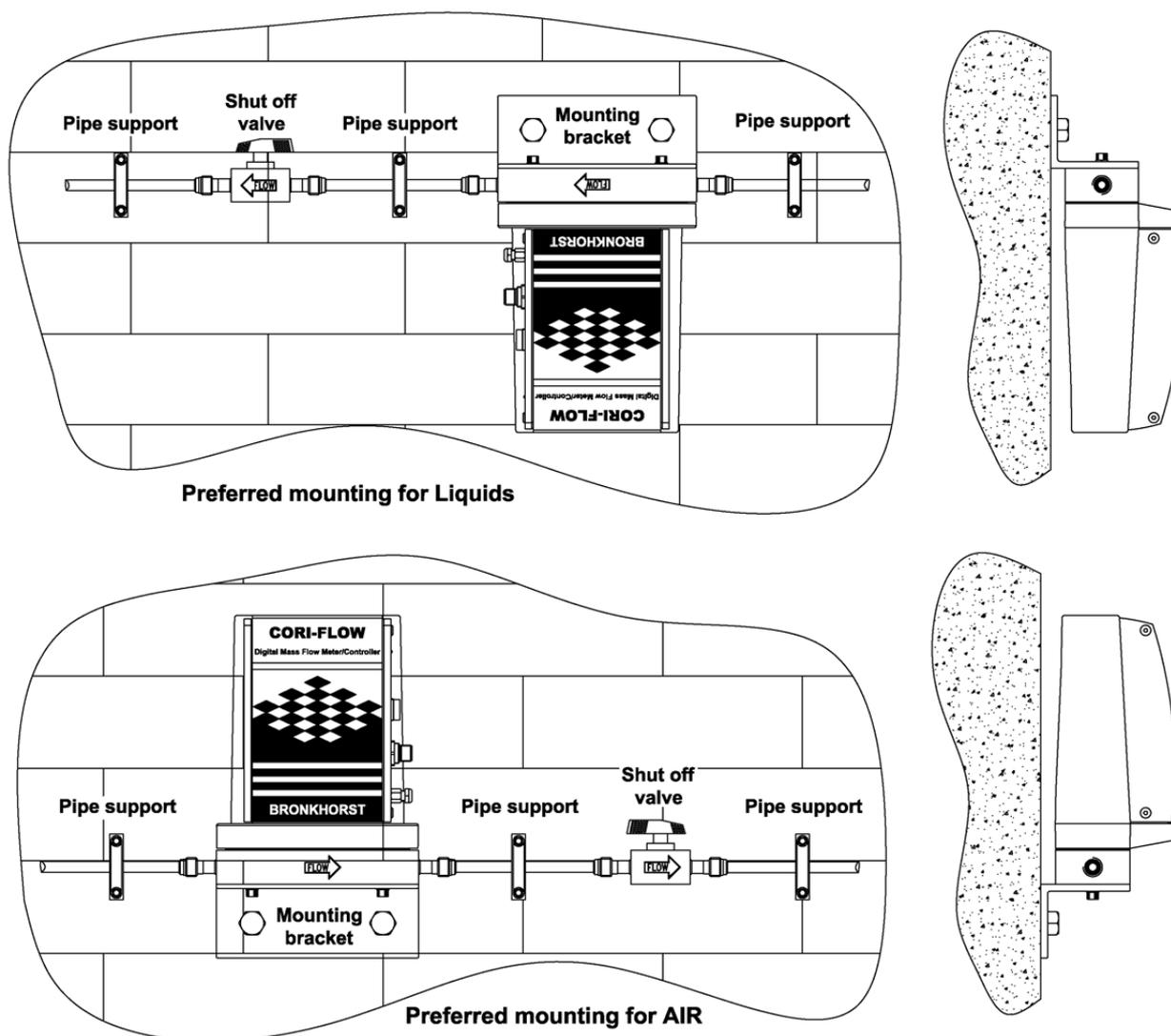
The first position, helps to remove gas bubbles out off the CORI-FLOW, the second prevents condensate collection. In order to remove gas bubbles during start-up, flushing with relatively high flow rate for some minutes is recommended.
