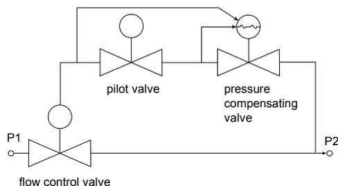
For high flow rates the pilot operated valve has been designed. A solenoid driven control valve controls the pressure difference across a piston, which lifts the main plunger.
