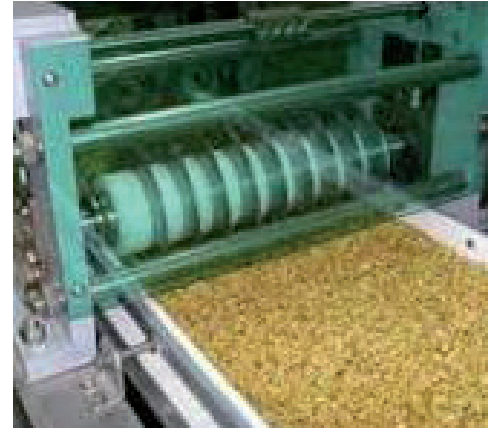
Roller showing extrusion of the product into long strips before cutting into bars.
